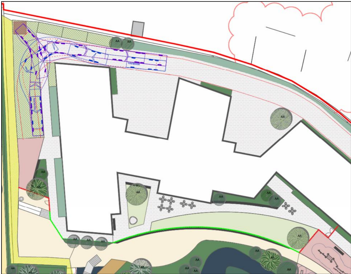
Figure 18.33 Fire tender tracking for Quarry PBSA
